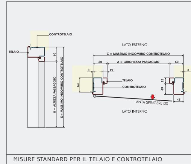
**MISURE PER IL TELAIO E C. T. STANDARD**
